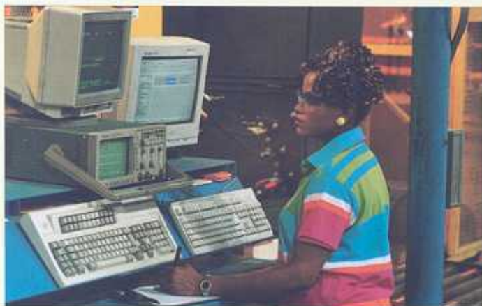
Computerized final test stations perform a complete series of electrical tests prior to shipment.
