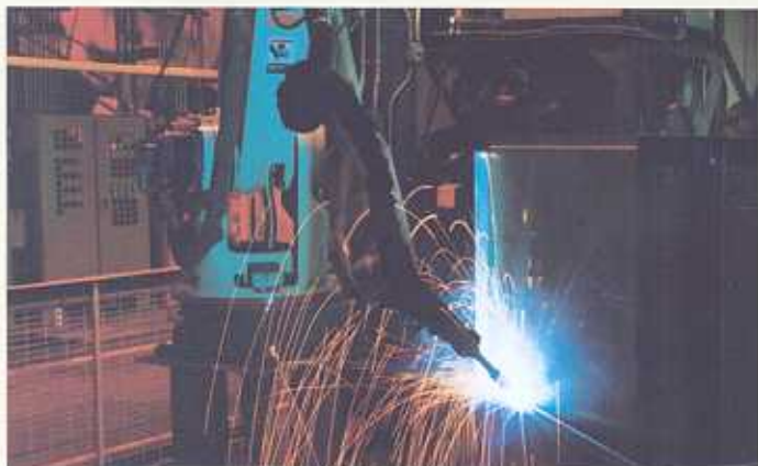
Automated and robotic welders perform 100% of all oil-compartment seam welds.
