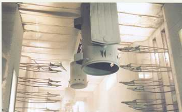
Electrostatically applied powder paint provides a durable, corrosion-resistant finish.
